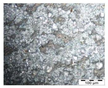
Figure 3: Morphology of Zn-40ZnO-0.5A composite coating
