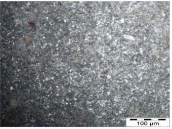
Figure 2: Morphology of Zn-20ZnO-1.0A composite coating
