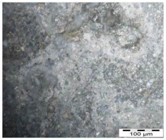
**Figure 4:** Morphology of Zn-40ZnO-1.0 A composite coating
