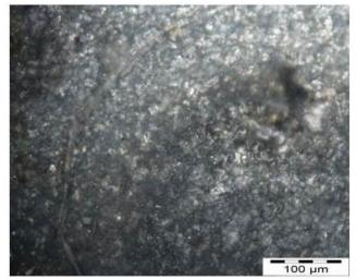
Figure 1: Morphology of Zn-20ZnO -0.5A composite coating
